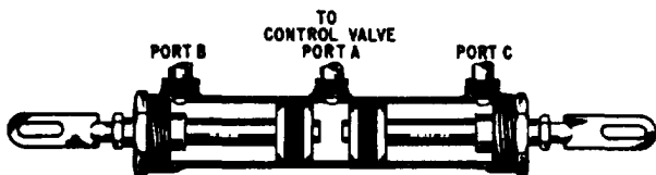
Figure 10-7.—Three-port, double-acting actuating cylinder.
